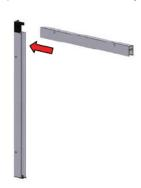
2.2.5. Insert the right guiding profile into the plastic corner component.
