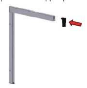
2.2.6. Insert the bottom corner component into the side profile.
