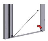
2.2.12. Test the polarity of the "magnet profile" then fix it to the "arrival profile".
